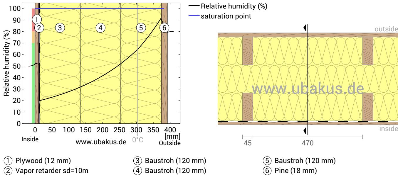
Notes: Calculation using the Ubakus 2D-FE method. Convection and the capillarity of the building materials were not considered. The drying time may take longer under unfavorable conditions (shading, damp / cool summers) than calculated here.
